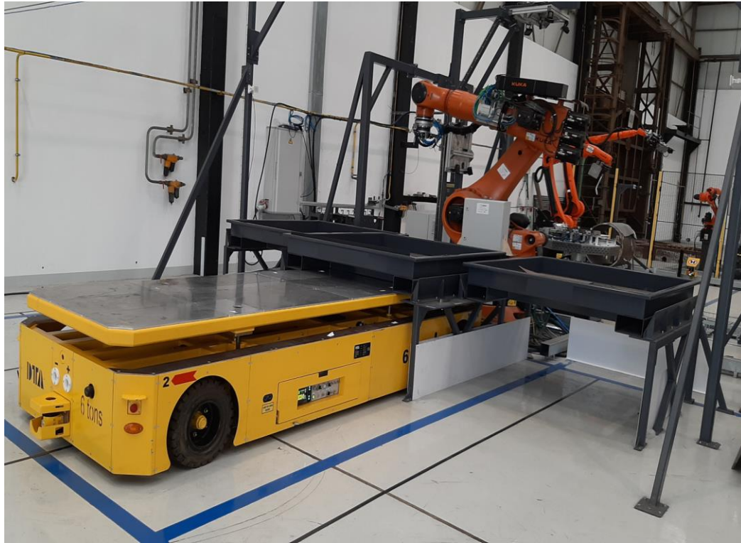
Transfer of materials into the welding cell
